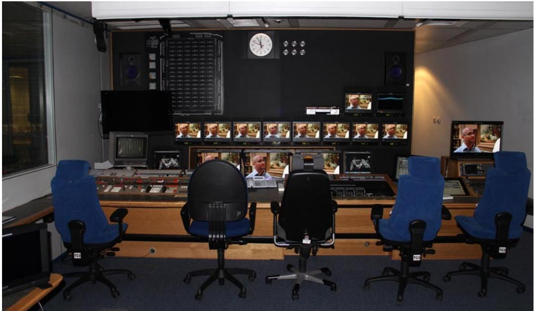
gigabit/s HD-SDI operation, adds ATG Danmon Projects Manager Dave Whitaker. "The main vision mixer was equipped with fibre-optic feeds from Sony HDC 1500 cameras. Other infrastructure incorporated included a Snell Cygnus router, Crystal Vision signal converters and additional glue equipment. Several of the existing production control desks were modified to incorporate additional equipment panels. We also reworked some of the Custom Consoles LCD-panel monitor stacks."
